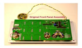
2. Make a chart of the Mic Config header wires on the front panel PCB, so you can keep track of which wire goes where. (five minutes)
